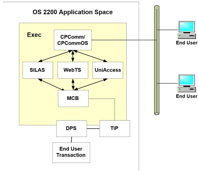
The diagram above shows the transaction flow between the user operating their terminal through to the application transaction program.
